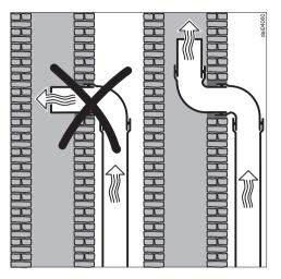
If the exhaust is ducted into an inactive flue, the air must be expelled parallel to the flow direction of the flue.
